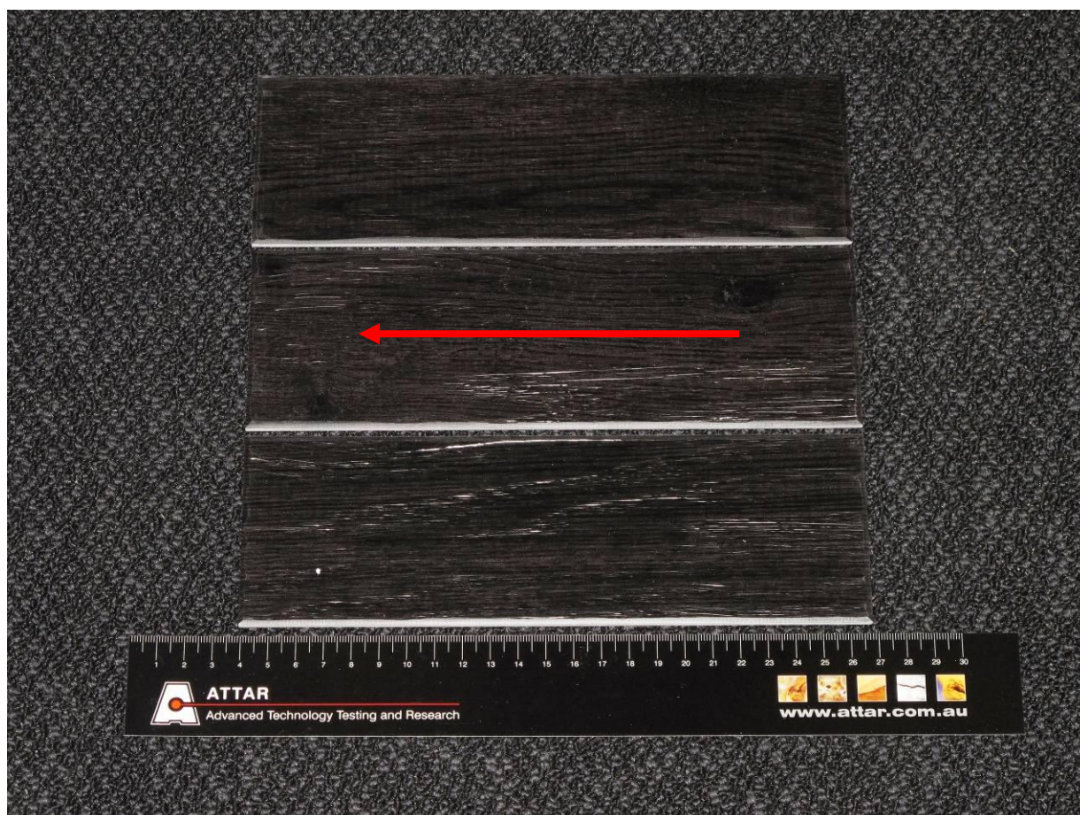
Figure. 1: Art Select - Parquet . Arrow indicates direction of testing
