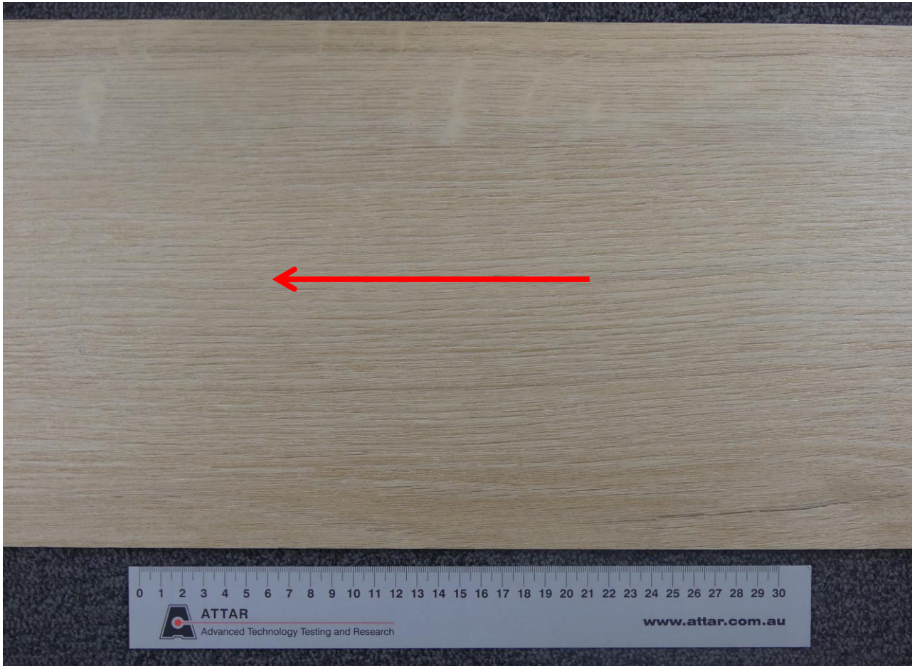
Figure 1: Karndean 1500mm x 250mm - DE092 Arrow indicates direction of testing
