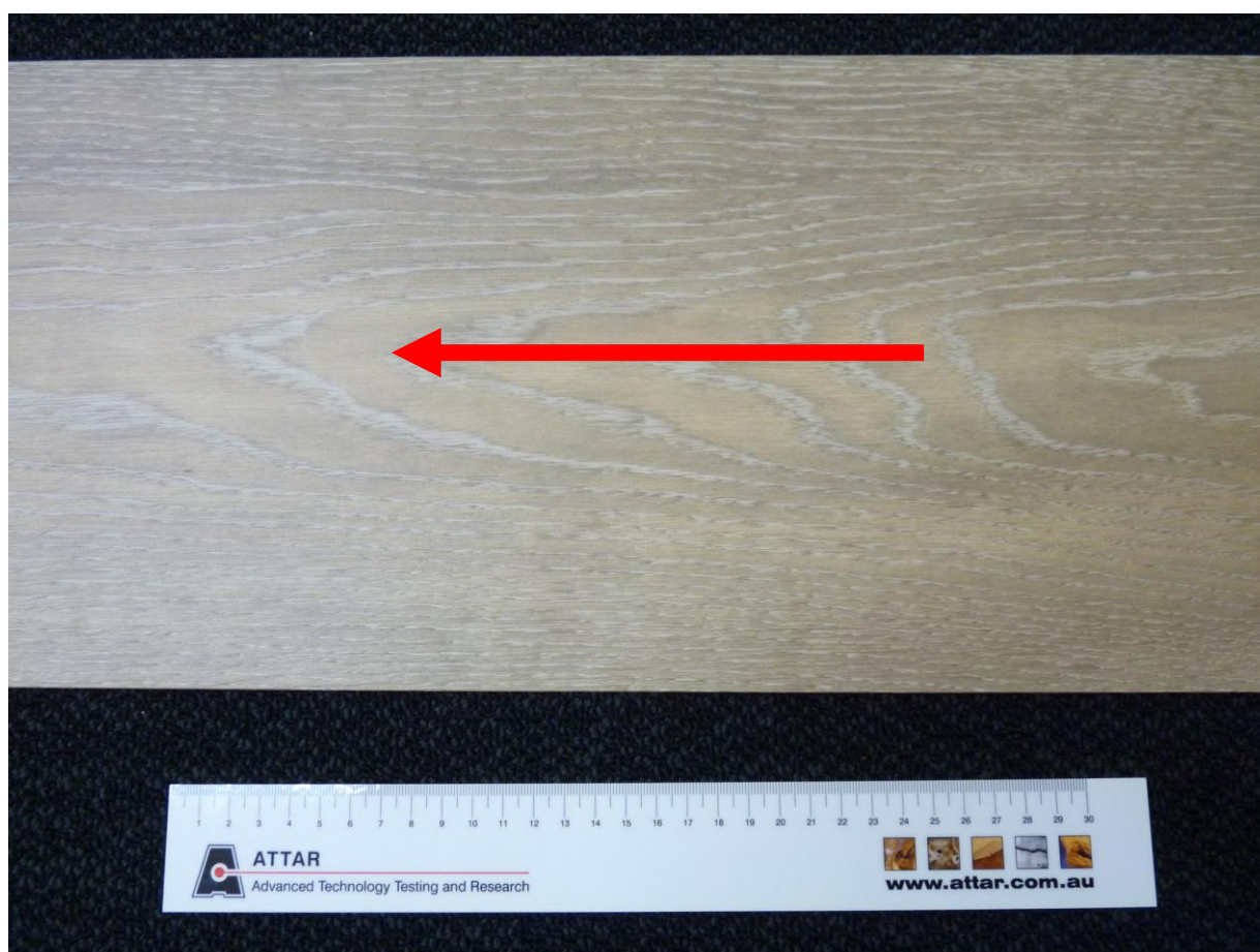
Figure 1: OPUS WP411-SR Vinyl Planks. Arrow indicates direction of test.
